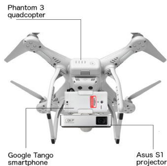
Figure 4. Drone configuration: Phantom 3 quadcopter, Asus S1 projector, and Google Tango.
