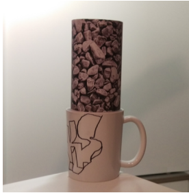
Figure 4: A printed marker was rolled up and placed inside the cup. This simple approach works as long as the walls of the cup are cylindrical in shape. Markings are a result of drawing “blocks” virtual contour (see Figure 6).
