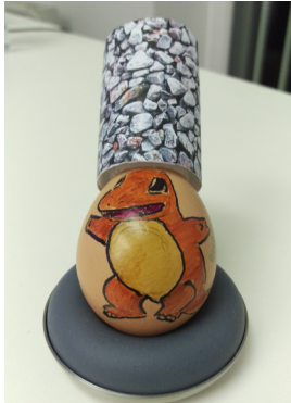
Figure 5: A printed marker was wrapped around cylindrically shaped object and glued on top of the egg. Markings on the egg are a result of drawing “animal” virtual contour (see Figure 7).
